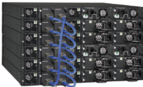
Figure 1: Up to 12 Brocade ICX 7450 switches can be stacked together using two full-duplex QSFP+ 40 Gbps ports that provide a fully redundant backplane with 160 Gbps of stacking bandwidth.
