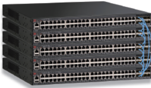
Figure 2: Up to 12 Brocade ICX 7250 Switches can be stacked together using up to four full-duplex SFP+ 10 Gbps ports for a fully redundant backplane with 80 Gbps of stacking bandwidth.
