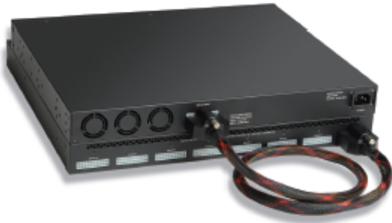
Figure 4: Rear view of the Brocade ICX-EPS 4000 connectivity.
